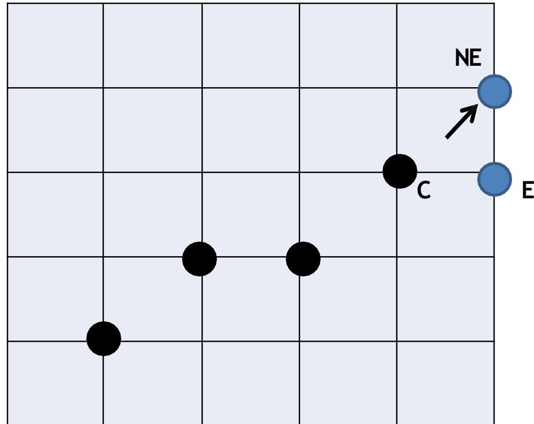
Next pixel is chosen (from E or NE) to build the line successively
