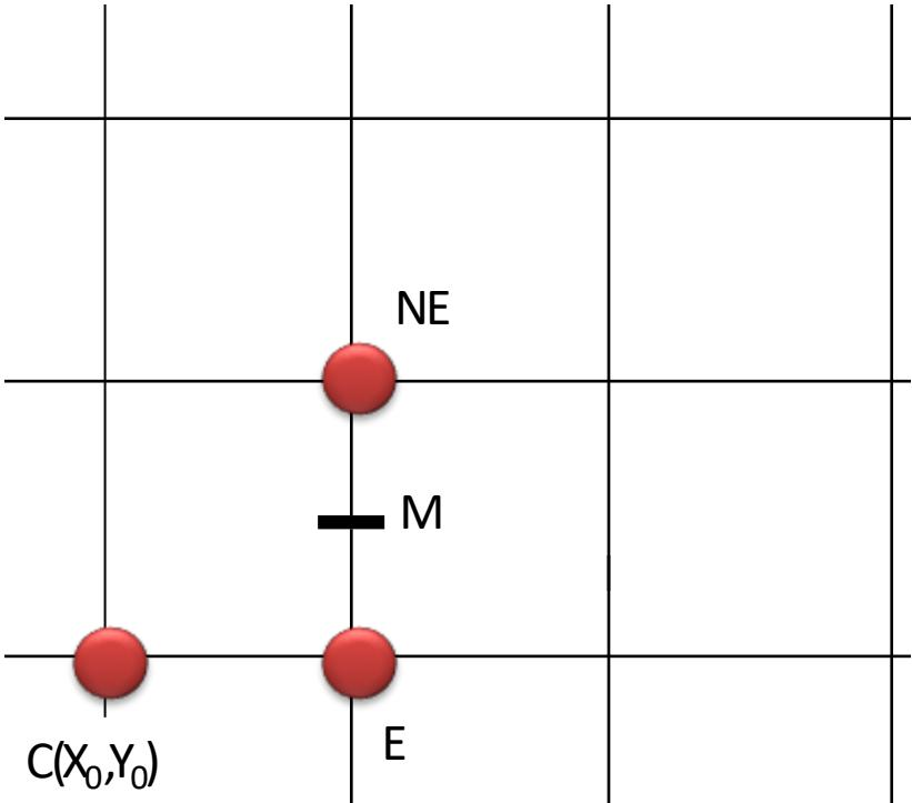
$$\begin{aligned}d_{\text{INIT}} &= F(M) \\&= F(X_0 + 1, Y_0 + 0.5) \\&= a(X_0 + 1) + b(Y_0 + 0.5) + c \\&= aX_0 + a + bY_0 + 0.5b + c \\&= aX_0 + bY_0 + c + a + 0.5b \\&= (aX_0 + bY_0 + c) + a + 0.5b \\&= F(X_0, Y_0) + a + 0.5b \\&= a + 0.5b \\&= dy - \mathbf{0.5}dx\end{aligned}$$
