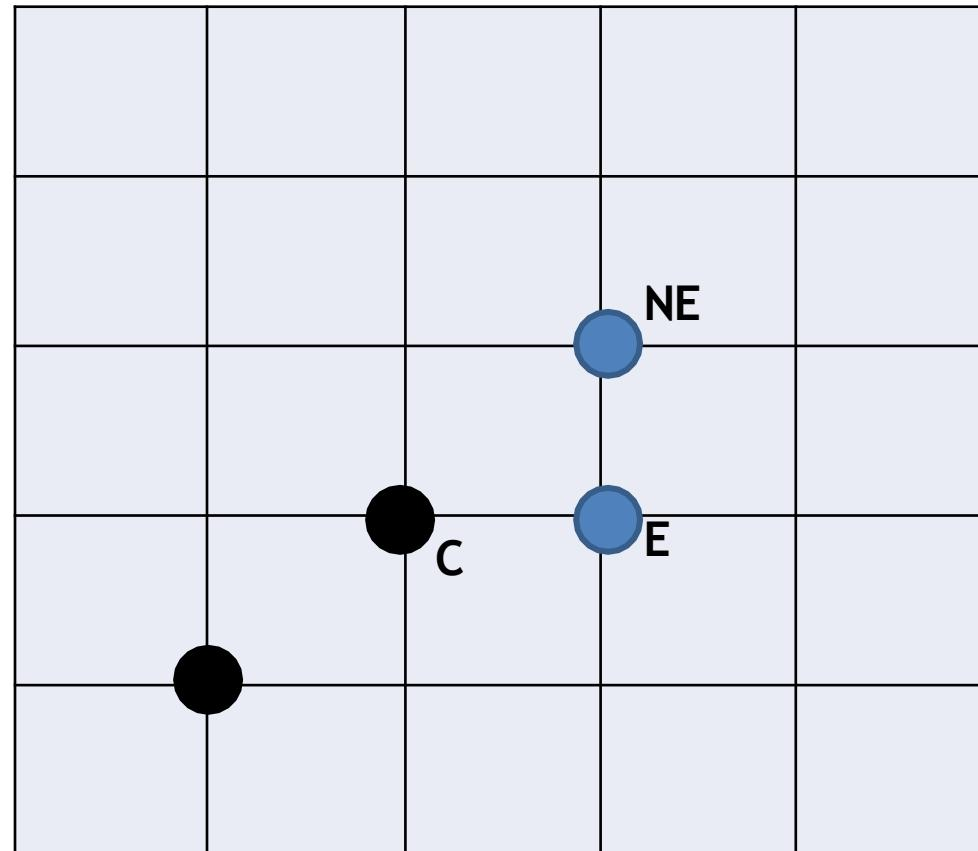
Next pixel is chosen (from E or NE) to build the line successively
