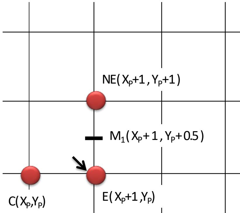
$$\begin{aligned}d_1 &= F(M_1) \\&= F(X_p+1, Y_p+0.5) \\&= a(X_p+1) + b(Y_p+0.5) + c\end{aligned}$$
