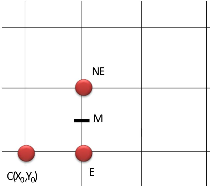
$$\begin{aligned}d_{\text{INIT}} &= F(M) \\&= F(X_0 + 1, Y_0 + 0.5) \\&= a(X_0 + 1) + b(Y_0 + 0.5) + c \\&= aX_0 + a + bY_0 + 0.5b + c \\&= aX_0 + bY_0 + c + a + 0.5b \\&= (aX_0 + bY_0 + c) + a + 0.5b \\&= F(X_0, Y_0) + a + 0.5b \\&= a + 0.5b \\&= dy - 0.5dx\end{aligned}$$
